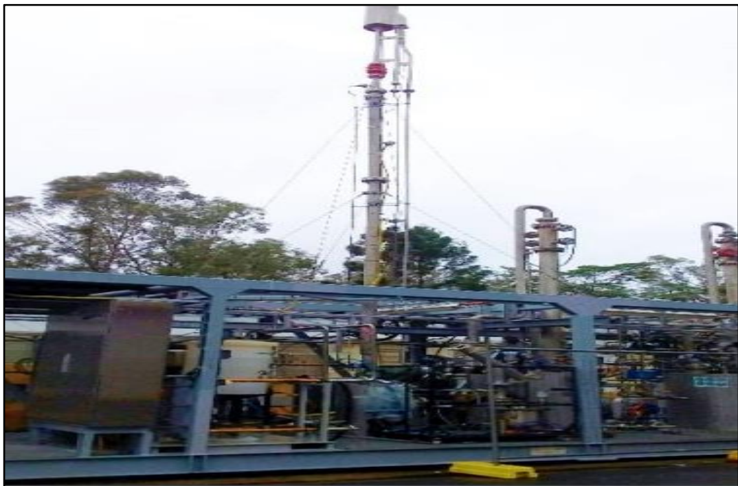
Figure 7: 1350 Kg/d hydrogen production module. Source: Synergen Met Pty Ltd website
