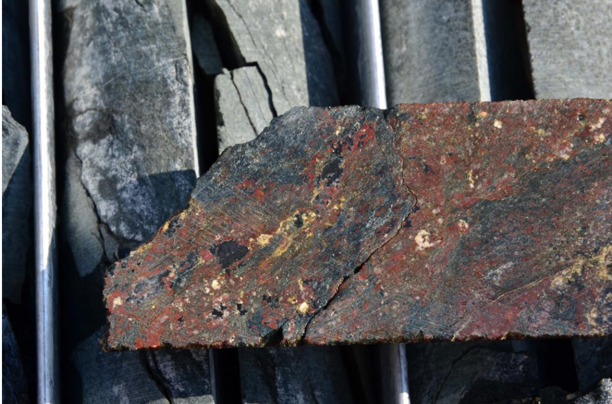
High Grade Breccia - Caramal - Hematite/Chlorite Altered Wallrock (Red), Uranium Mineralisation (Dark)
