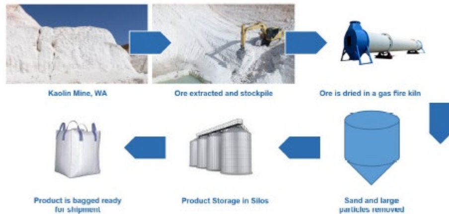
FIGURE 6 THE DRY PROCERSS FOR MAKING K99 PRODUCT
