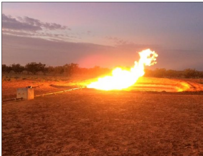
Figure 16: Gas flare from testing of Tamarama1.
