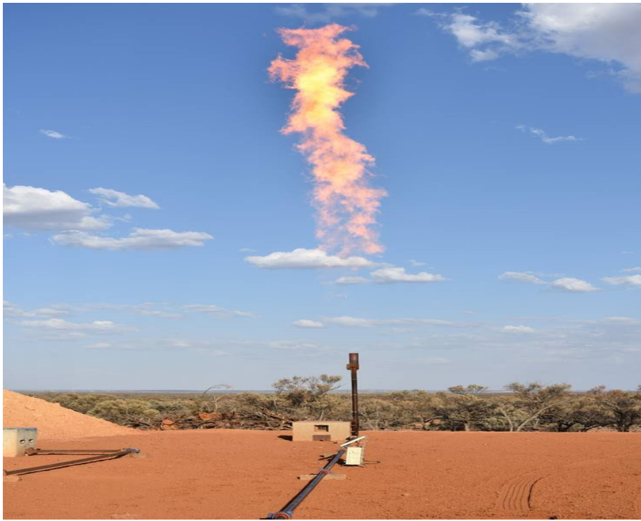
Figure 14: Gas Flare from testing of Tamarama 2
