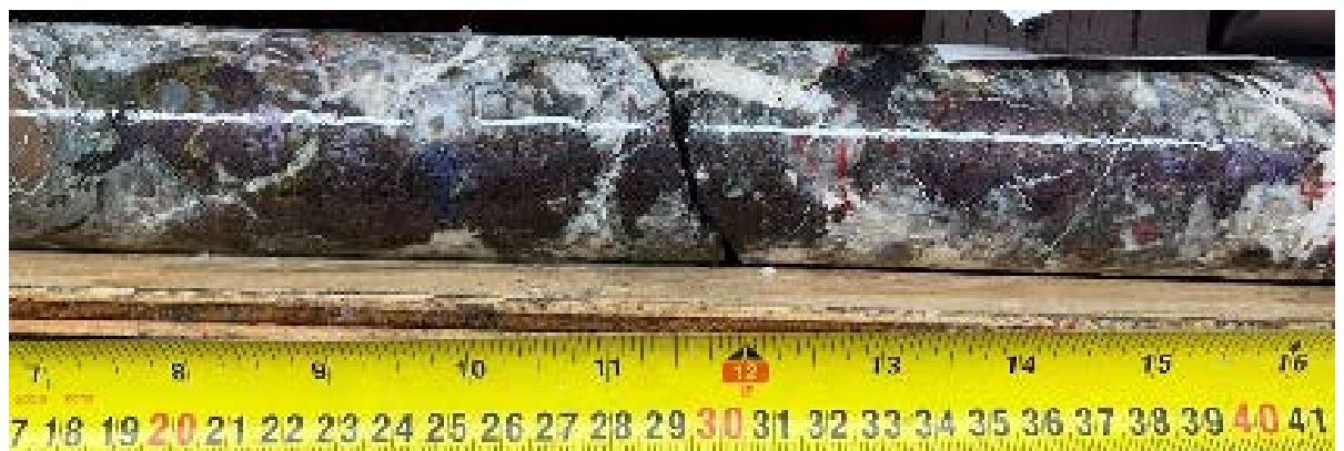
Figure 13: Bornite Hills hole BNH003, 83.7 m to 83.9 m, showing bornite and chalcopyrite breccia-hosted mineralisation: Source: White Cliff Minerals
