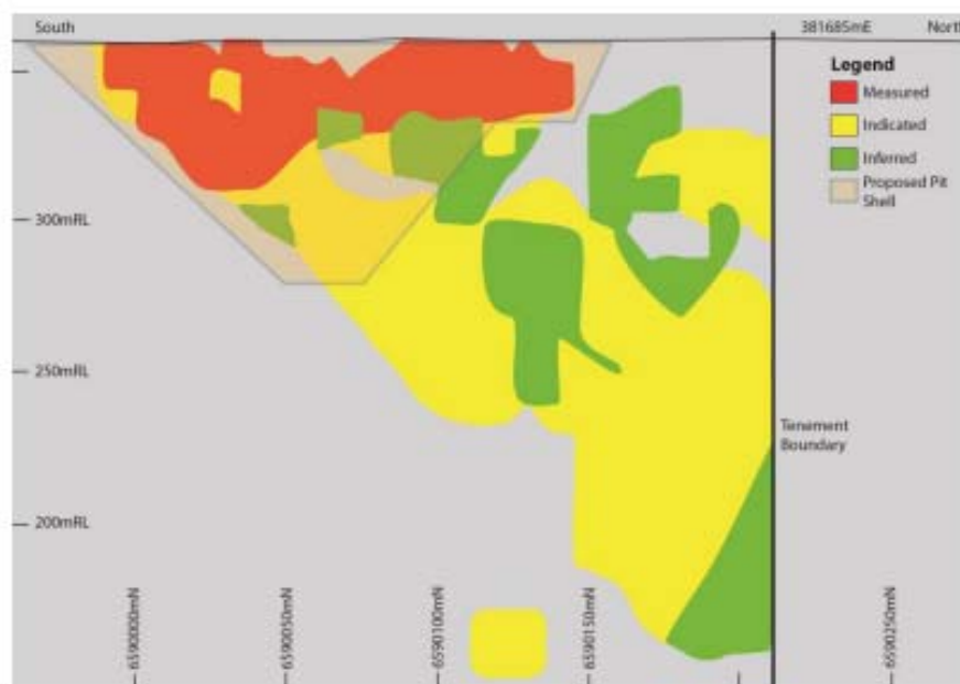
Figure 2: Long Section of Cannon Resource by Category on Section 381685mE with Pit Shell Source: Southern Gold Ltd
